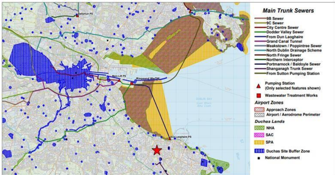
Figure 16.4: Foul Catchments to Ringsend WwTP.
